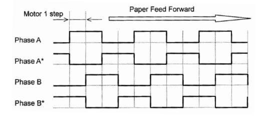
There are four different positions for the stepper motor. The driving is bipolar and can be achieved with circuits like: the Rohm BA6845FS, the Sanyo LB1846, LB1848, or LB11948T which offer a PWM current control. Please refer to the IC's data sheet for further information. It is recommended not to exceed 0.2V like voltage drop in the stepper motor driver circuit.
